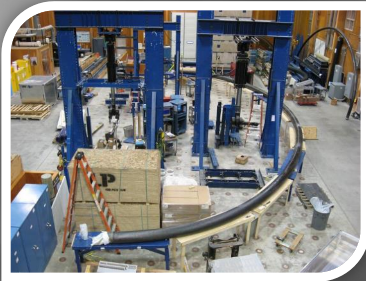
Manufacturing of 60' Span Arch
