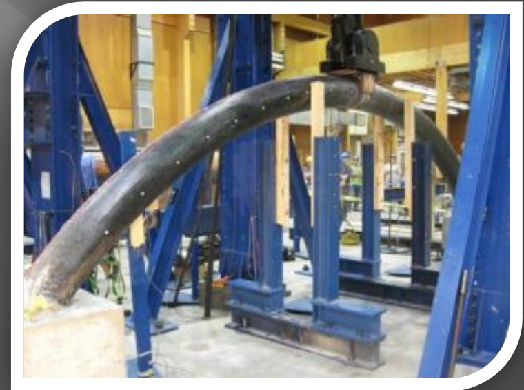
Arch Structural Testing
