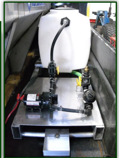
50 gal. tank, clean out port, filter, pump, return line, supply line and two nozzles: \$400-\$500 invested
