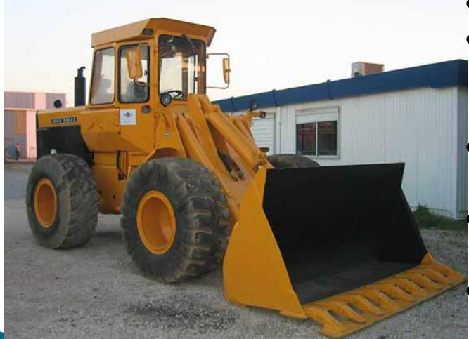
•131 hp Tipping cap. 16,000 lb. BUCKET 2.75 Weight 25,220 lb. Dump Clearance 9'2"
