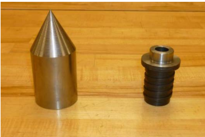
Cone casing and adaptor used to push the sensors to depth of interest
