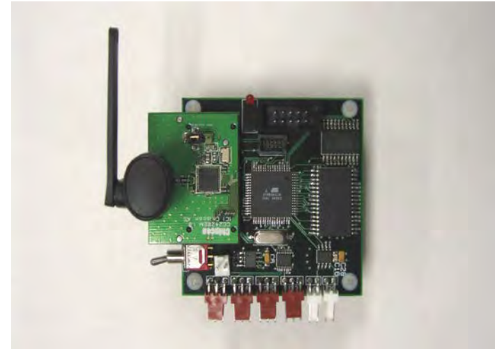
Wireless sensor node.
