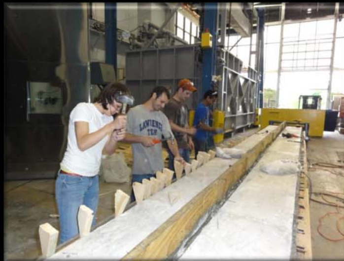
Removing sides of formwork
