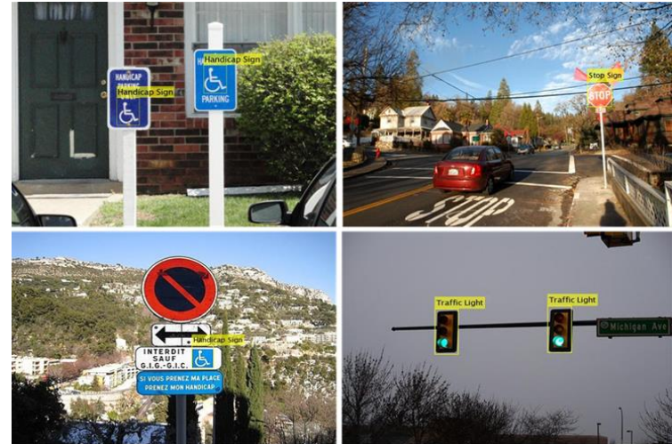
Detection of asset data in training imagery – stop signs, handicap signs, traffic lights
