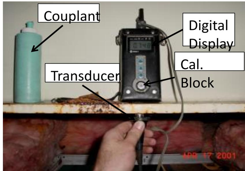
Typical technology uses a single transducer and a digital display showing thickness measurement
