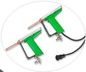
Current flows between prods (running current magnetizes material)
