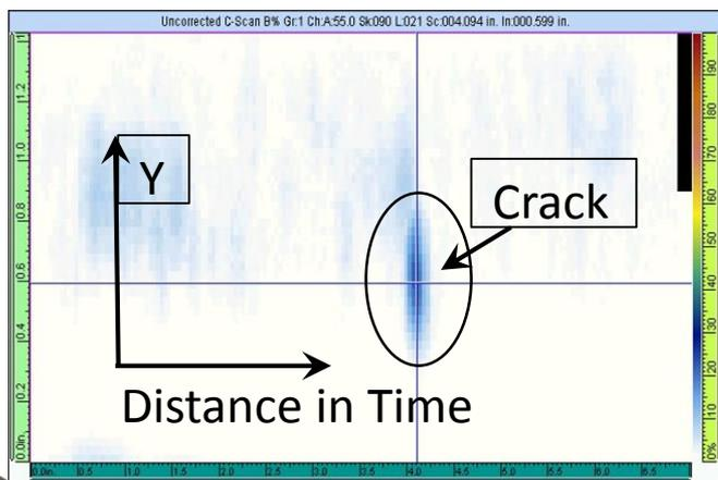
C-scan image of crack signals
