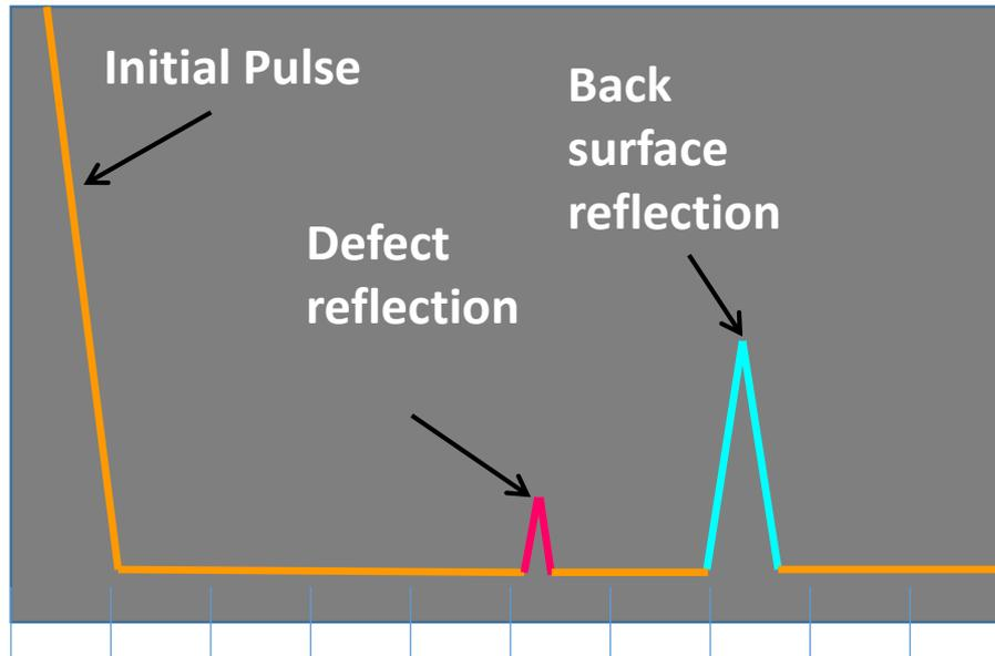
Note: A crack normal to the beam path reflects more energy than a crack that is skewed
