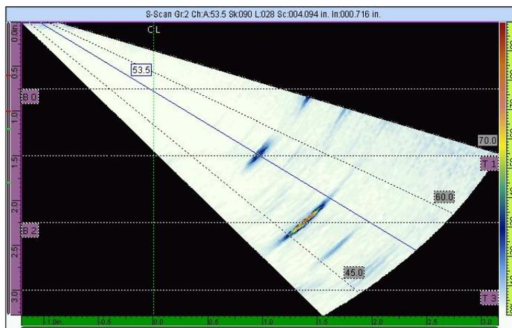
S-scan image of crack signals
