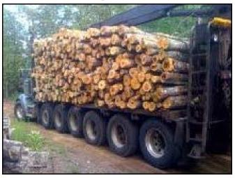
Michigan limits the maximum number of axles to eleven and per-axle load restrictions have resulted in a maximum gross vehicle weight of 164,000 pounds.
